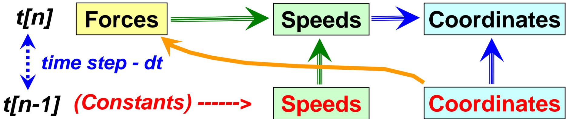
The speeds and coordinates at  $t[n-1]$  are copied from the speeds and coordinates at  $t[n]$ . Therefore the formulas are using their old results to calculate the results in an infinite loop.
